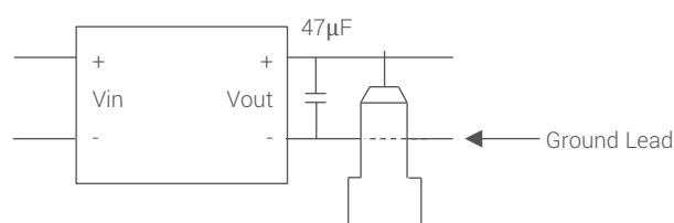
Measured with 20MHz bandwidth and 47μF ceramic capacitor.
