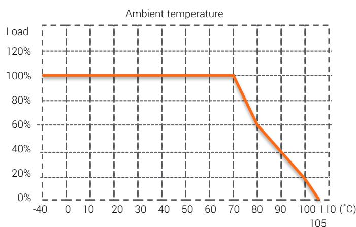
The de-rating curve was measured at 110V input in chamber with natural convection.
