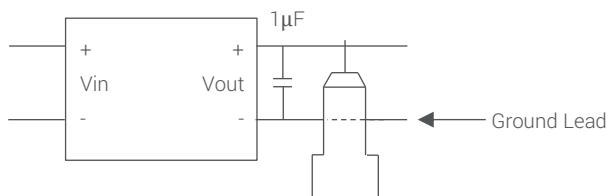
Measured with 20MHz bandwidth and 1μF ceramic capacitor
